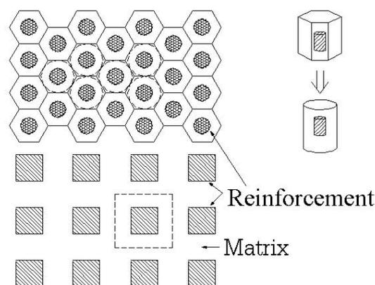
Fig. 2 The axisymmetric unit cell for modelling PRMMCs
