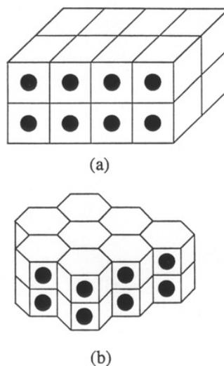
**Fig. 1** Periodic inclusion packing arrangement often used in micromechanical investigations of PRMMCs (a) cubic and (b) hexagonal
