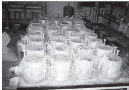
Fig. 4 Curing samples for CBR test
