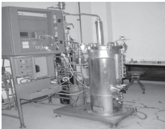
Fig. 2 A 50-L stirred-tank reactor for NPV production.
