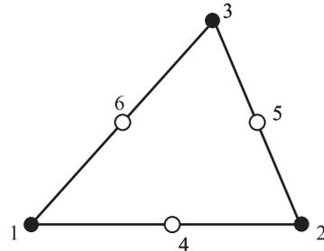
Fig. 1 Element with nodeless variables and its connectivity.
