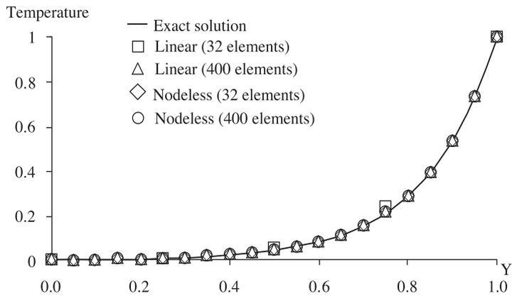
**Fig. 6** Temperature distribution along y axis at x = 0.25
