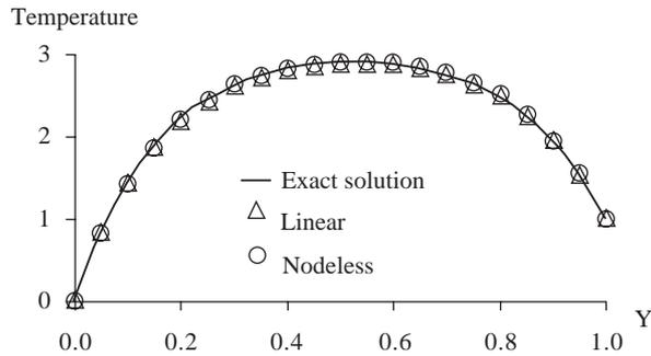
**Fig. 11** Temperature distribution along  $y$  axis at  $x = 0.25$  of rectangular plate with sinusoidal temperature at top edge and internal heat generation.
