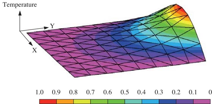
**Fig. 3** Temperature distribution on rectangular plate.
