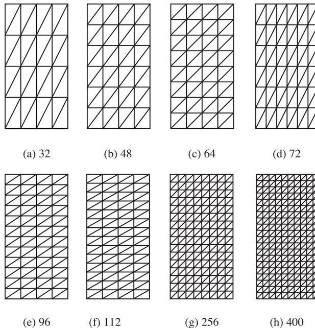
**Fig. 4** Finite element number of rectangular plate.
