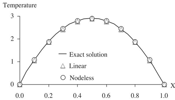
**Fig. 10** Temperature distribution along  $x$  axis at  $y = 0.5$  of rectangular plate with sinusoidal temperature at top edge and internal heat generation.
