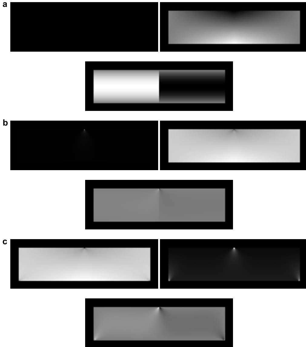
Fig. 7 Maps of \sigma_{xx} , \sigma_{yy} , and \tau_{xy} generated with the ratio l/c = 4.00 exploiting (a) the Bernoulli-Euler Theory, (b) the Wilson-Stokes theory, and (c) the Durant-Garwood theory. Read horizontally and vertically.
