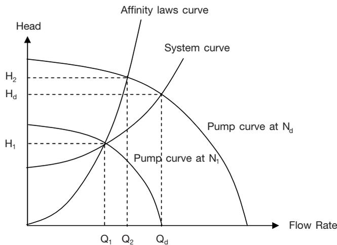
**Fig. 2** Illustration of a method to find the pump speed ( $N_1$ ) to deliver the required fluid flow rate ( $Q_1$ ), given the system curve, the pump performance curve, and the design flow rate
