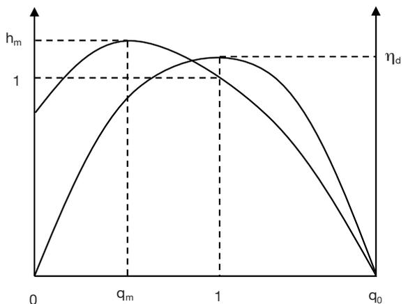
Fig. 3 Head curve and efficiency curves of the theoretical pump
