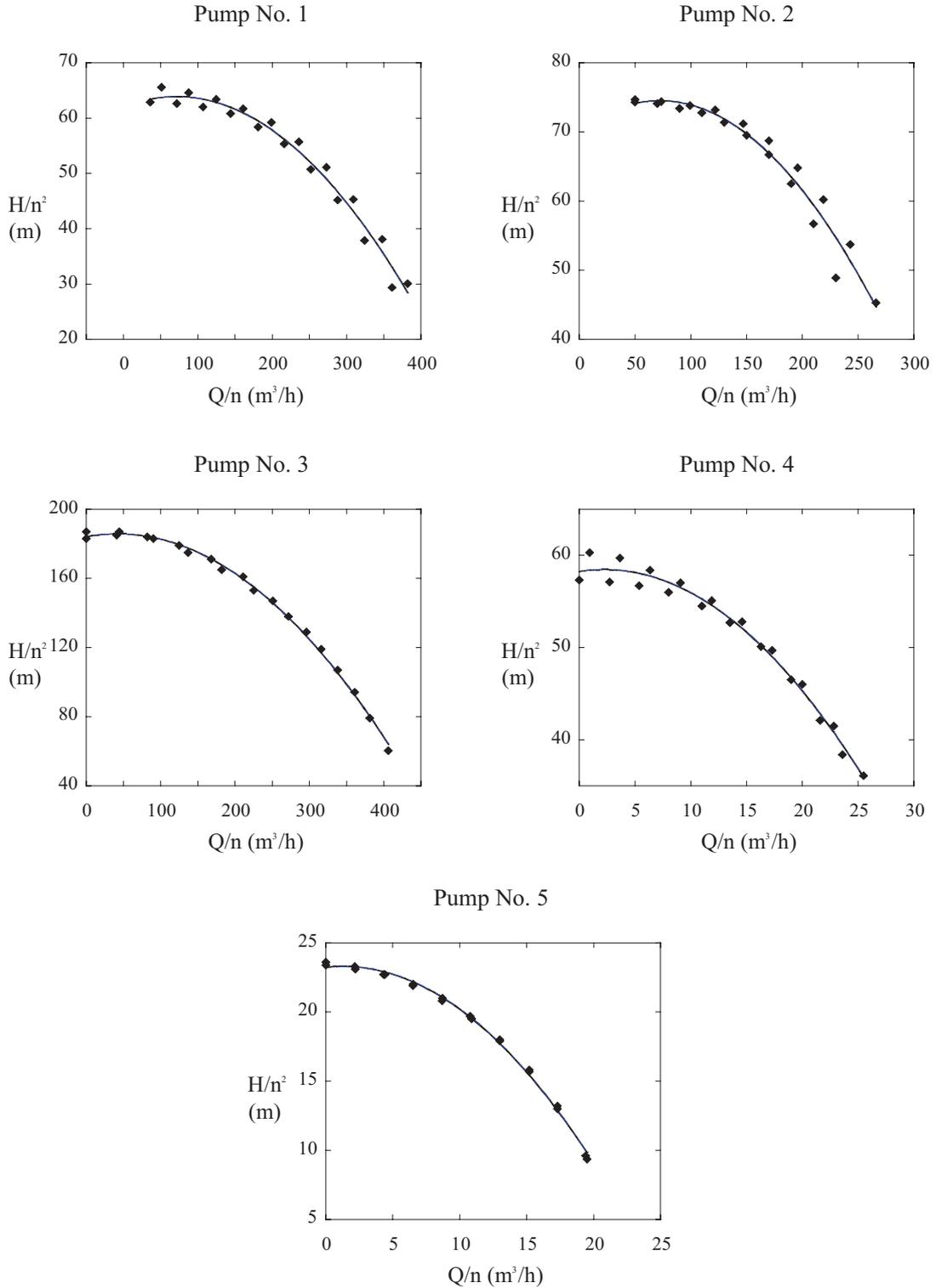
**Fig. 5** Comparison between data points extracted from head curves of 5 pumps and head curves of corresponding theoretical pumps
