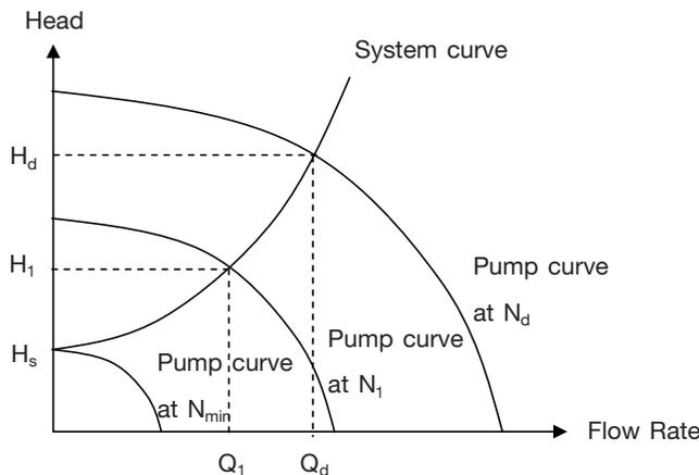
**Fig. 1** Demonstration that the existence of static head ( $H_s$ ) requires the pump speed to be at least  $N_{min}$ .
