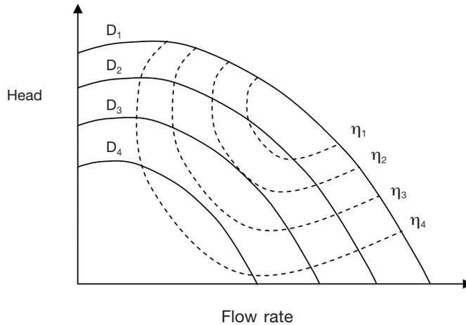
**Fig. 4** Pump performance curves at a constant pump speed provided by pump manufacturers
