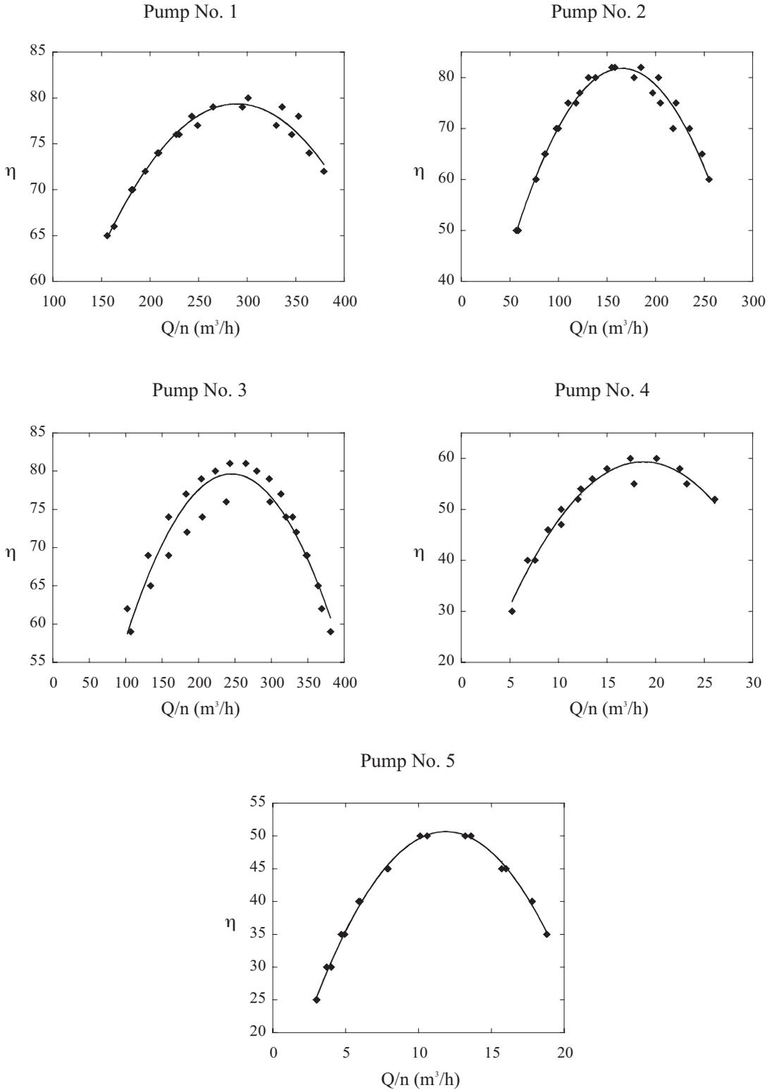
**Fig. 6** Comparison between data points extracted from efficiency curves of 5 pumps and efficiency curves of corresponding theoretical pumps
