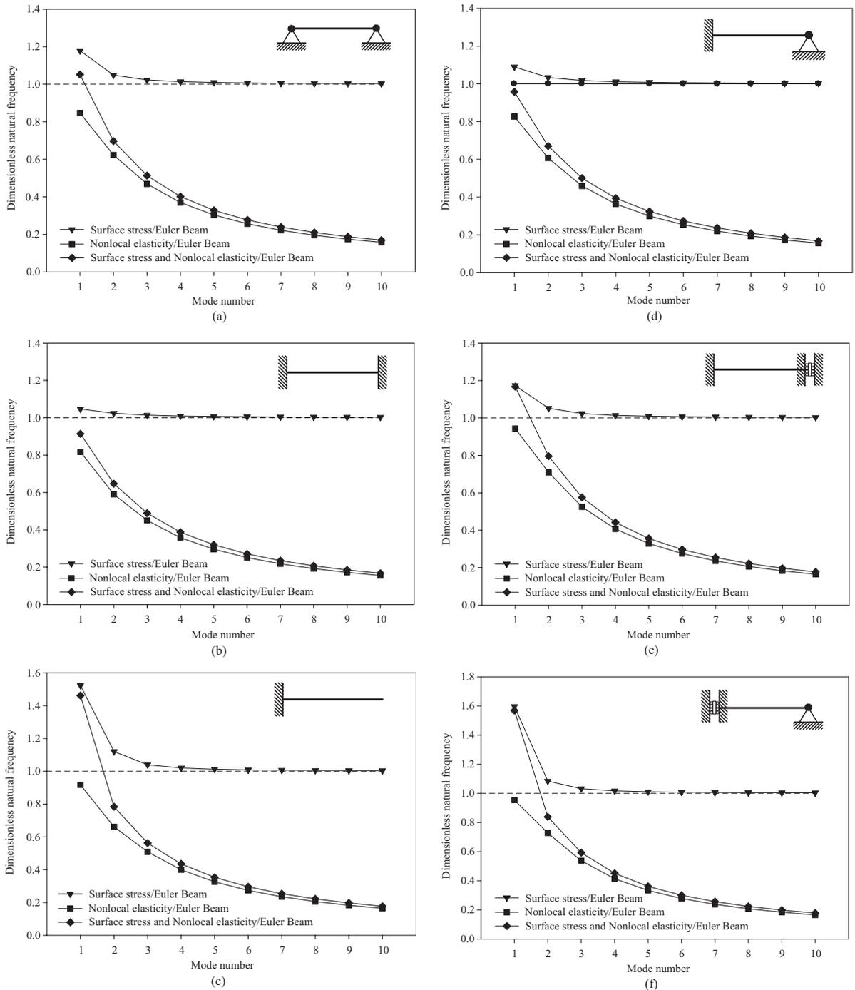
**Fig. 9** Variation of dimensionless natural frequency with surface stress and non-local elasticity effects for different boundary condition: (a) pinned-pinned, (b) clamped-clamped, (c) clamped-free, (d) clamped-pinned, (e) clamped-sliding, and (f) sliding-pinned.
