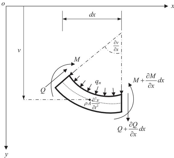
Fig. 2 Free body of an infinitesimal segment of nanobeams.
