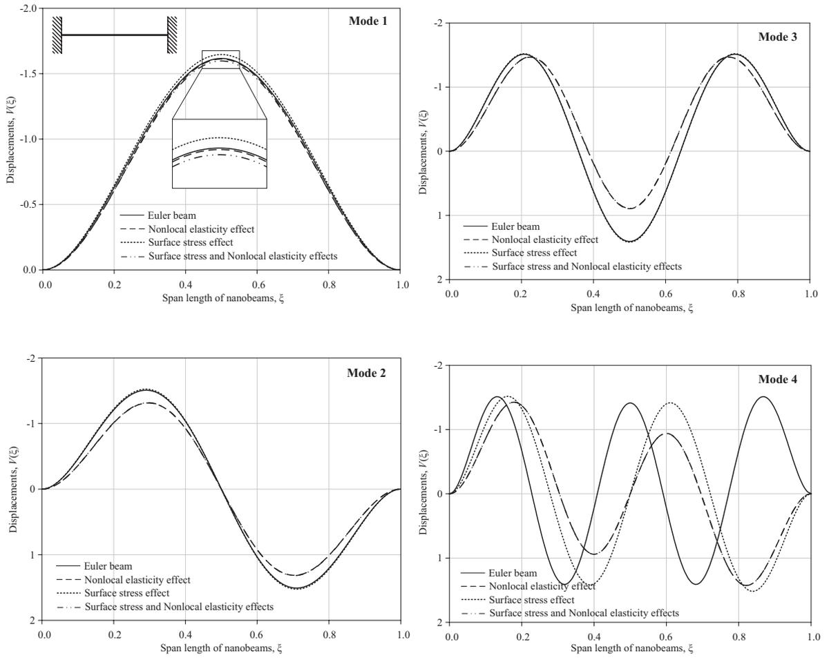
**Fig. 4** Variations of mode shapes of clamped-clamped nanobeams.
