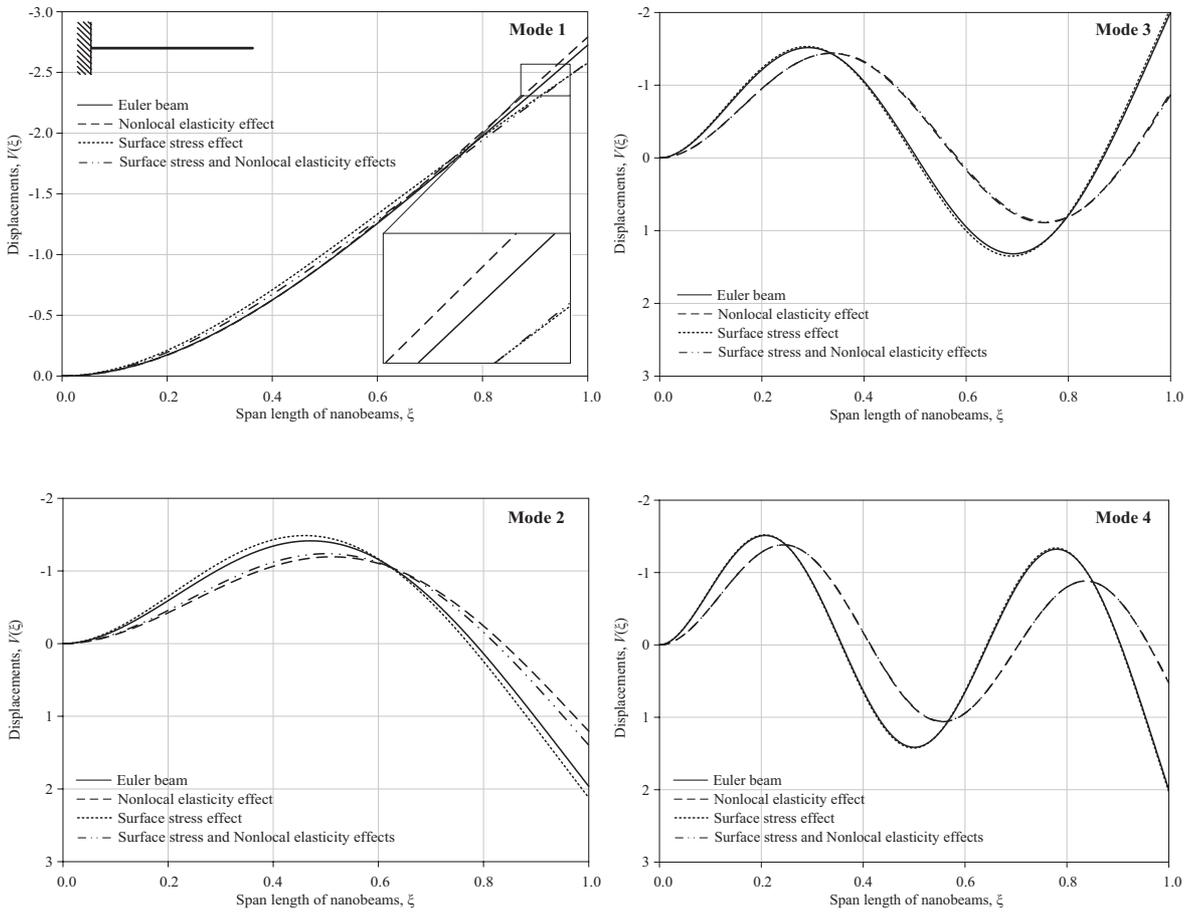
Fig. 5 Variations of mode shapes of clamped-free nanobeams.
