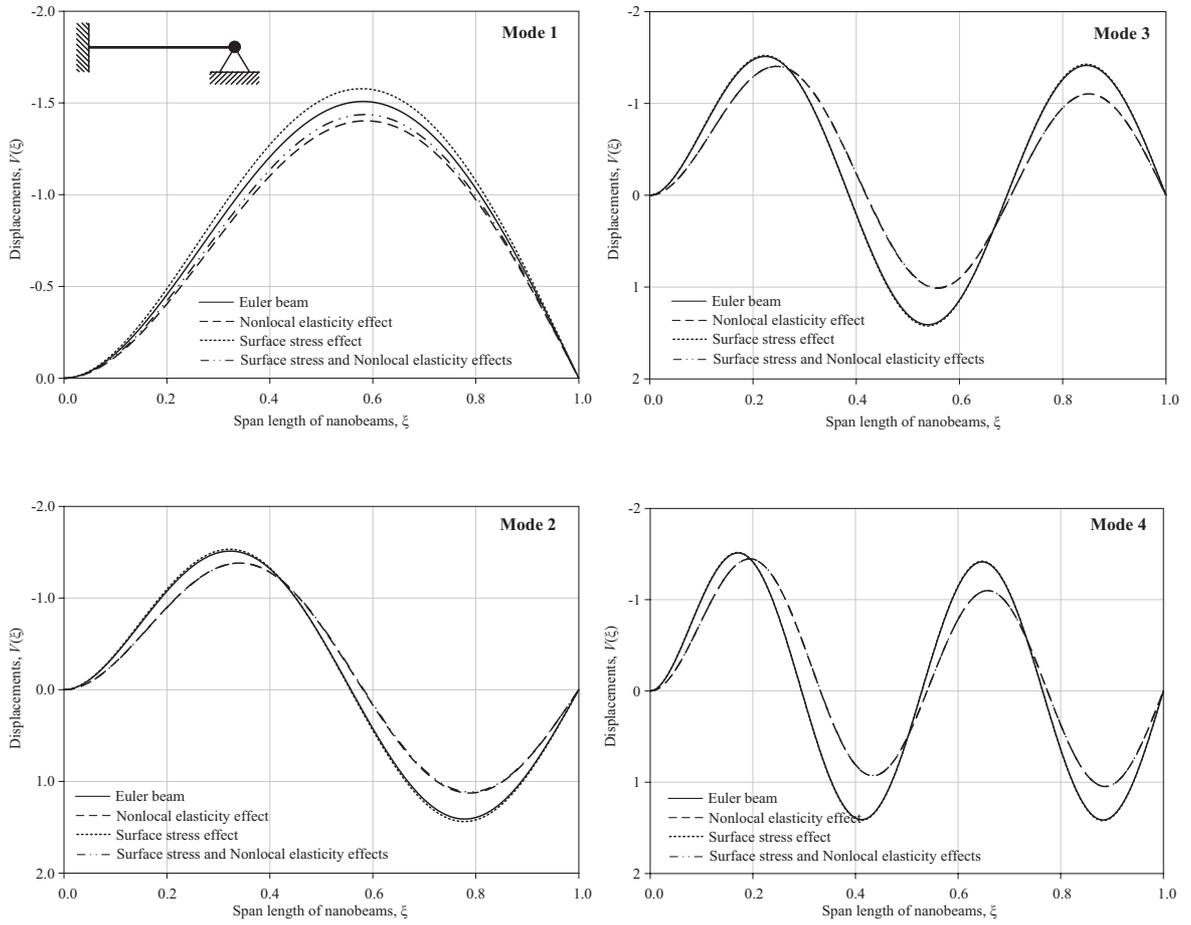
**Fig. 6** Variations of mode shapes of clamped-pinned nanobeams.
