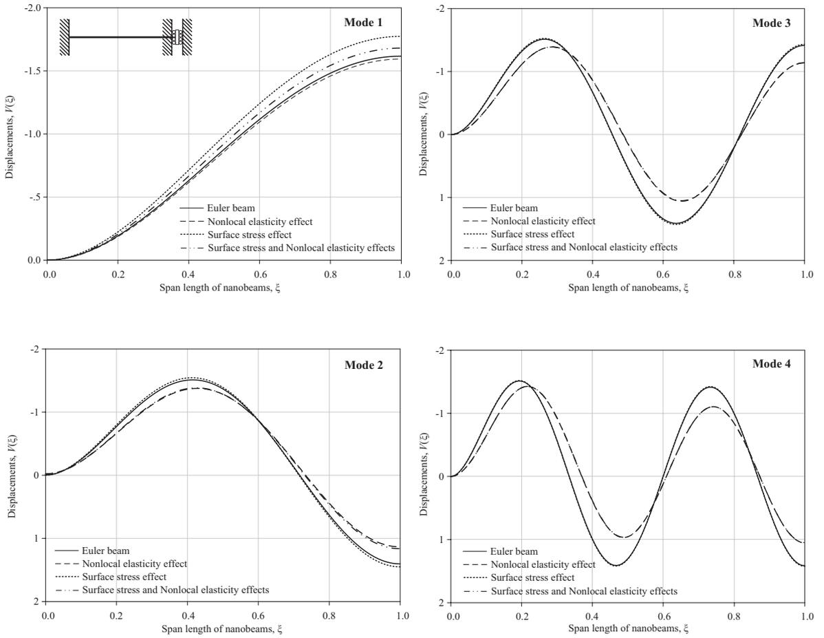
**Fig. 7** Variations of mode shapes of clamped-sliding nanobeams.
