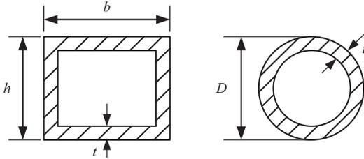
**Fig. 1** A rectangular and circular cross section of nanobeams with a surface layer.
