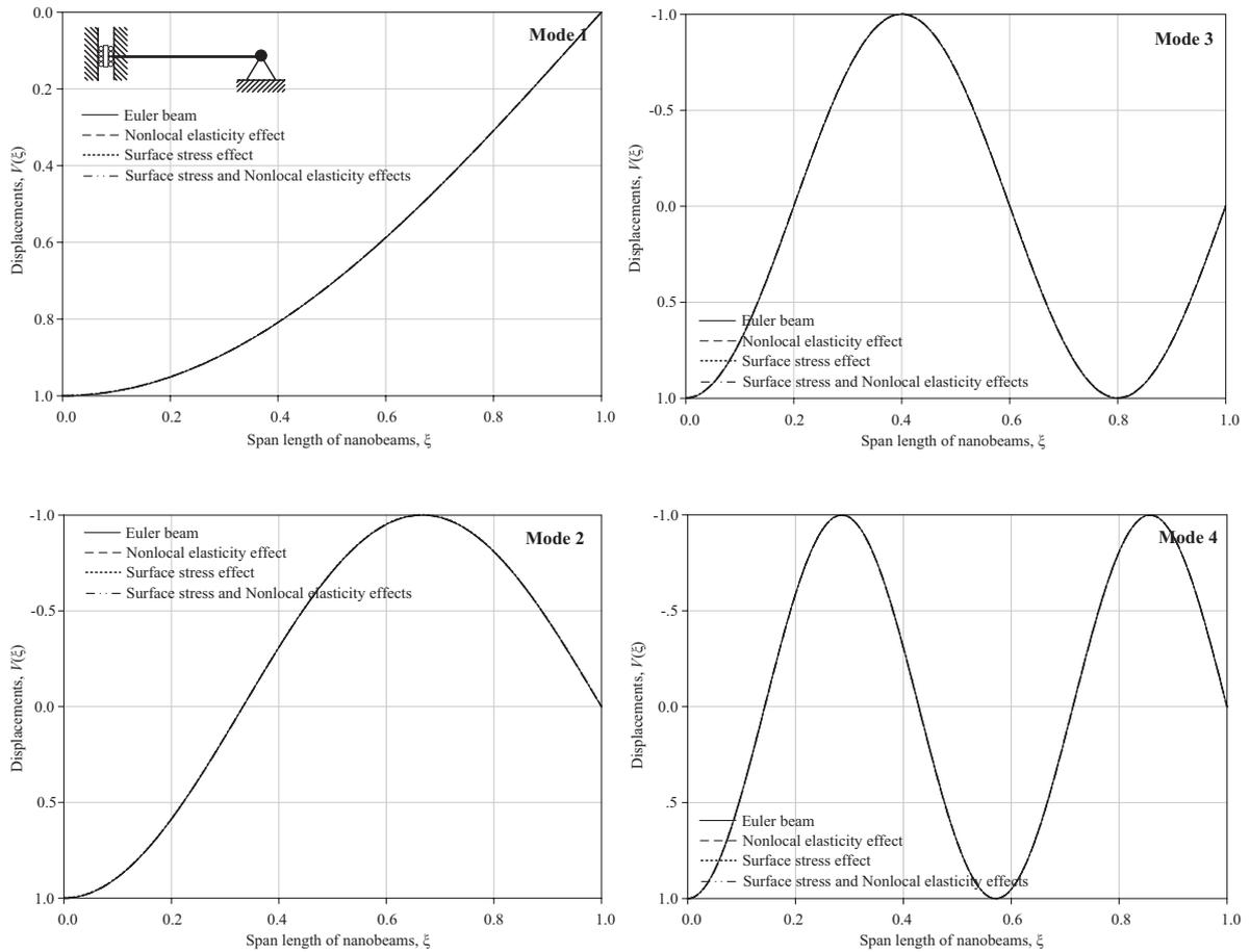
**Fig. 8** Variations of mode shapes of sliding-pinned nanobeams.
