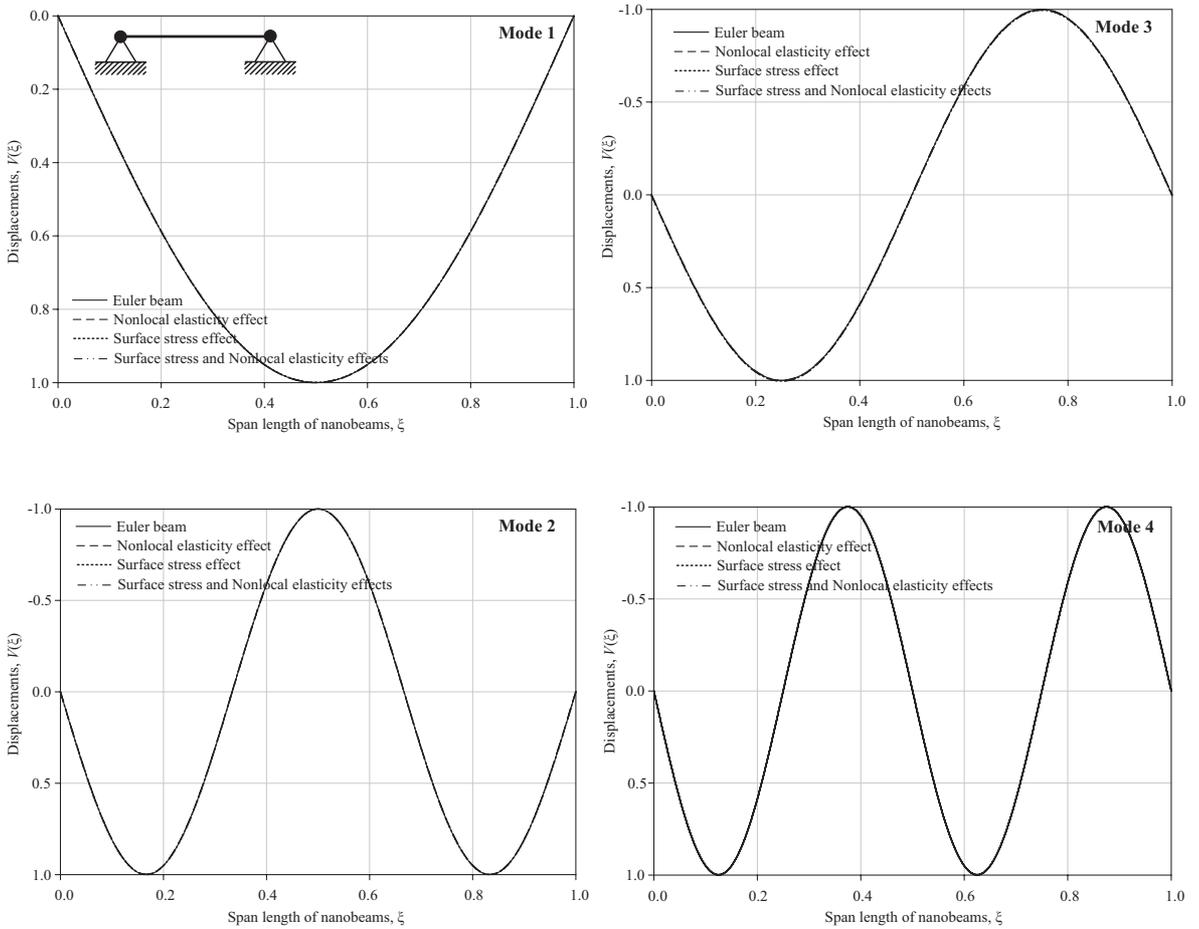
**Fig. 3** Variations of mode shapes of pinned-pinned nanobeams
