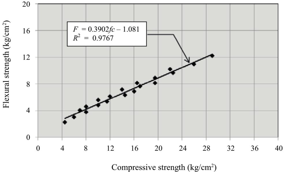
**Figure 8** Relationship between the compressive strength and flexural strength
