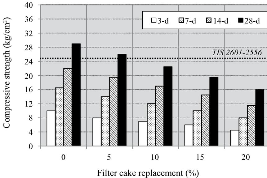
**Figure 6** Compressive strength development of CLC mixtures as a function of time
