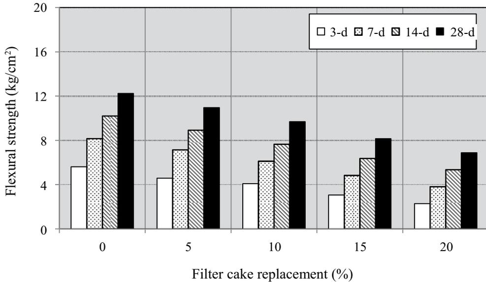
**Figure 7** Flexural strength development of CLC mixtures as a function of time
