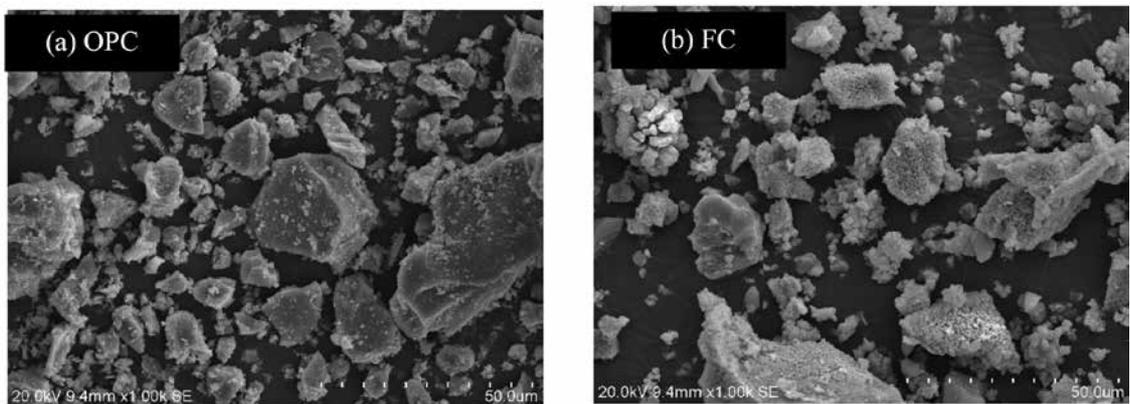
**Figure 2** SEM images of (a) OPC and (b) FC (magnification ~1000×)
