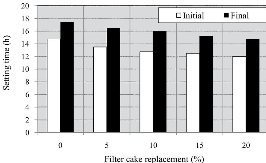
**Figure 5** Setting time for CLC mixtures
