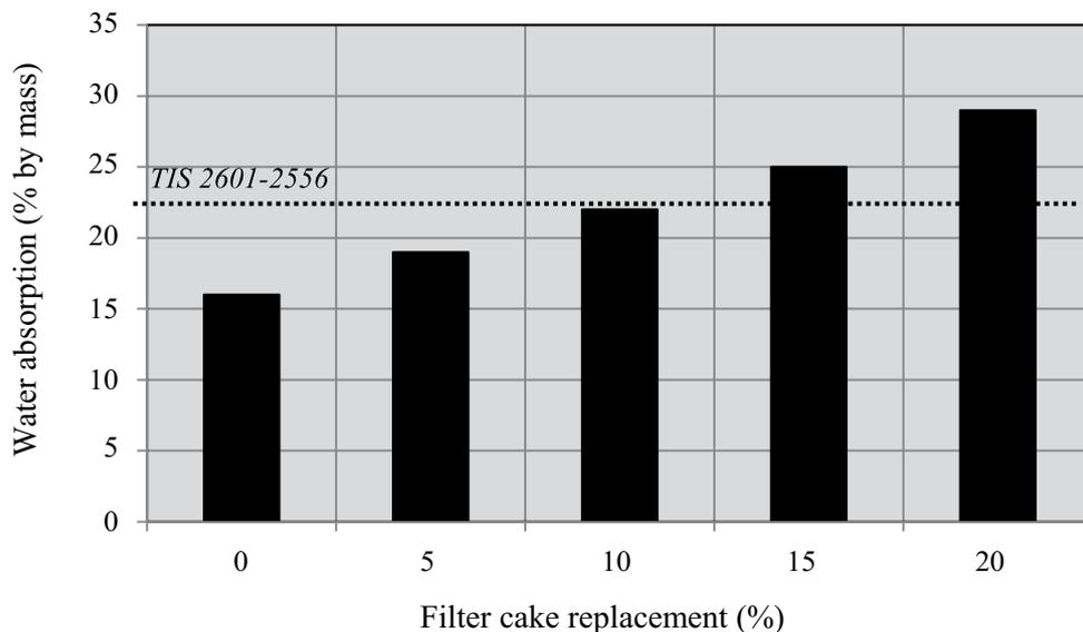
**Figure 10** Water absorption of CLC at 28 days
