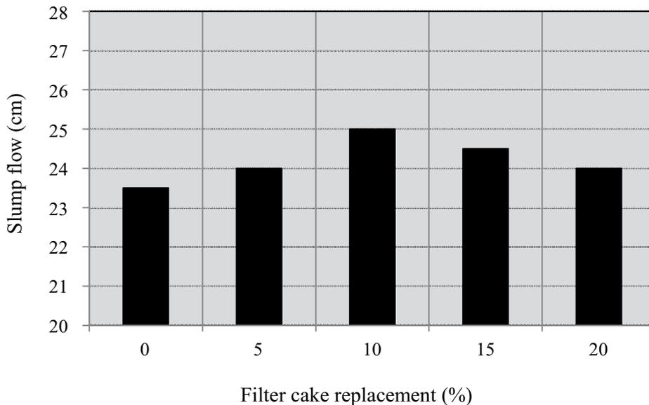
Figure 4 Slump flow for CLC mixtures
