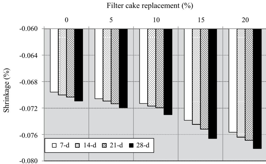
**Figure 9** Shrinkage of CLC mixtures as a function of time
