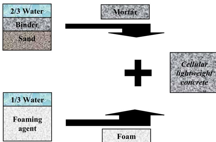
**Figure 3** Pre-foaming method diagram for foamed concrete [6]
