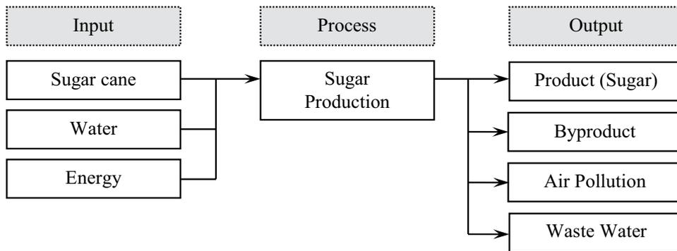
**Figure 1** Inputs and outputs of the production process of sugar derived from sugarcane [1]
