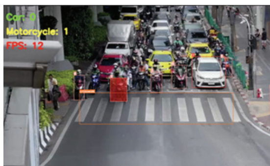
Figure 4 Pedestrian crosswalk violation detection and offender counting using DeepSORT, where the largest orange bounding box indicates the pedestrian crosswalk and red shaded boxes indicate vehicles violating the pedestrian crosswalk
