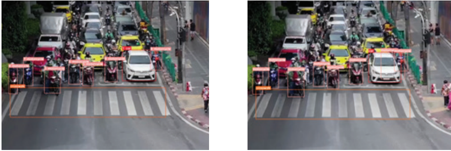
Figure 6 Examples of predicted bounding boxes obtained from DeepSORT tracking (a) and manual tracking (b)
