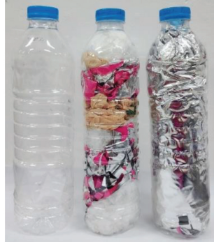
Figure 1 Empty PET bottles (left), APB-filled PET bottles (center), and LAF-filled PET bottles (right)
