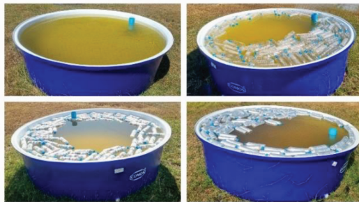
Figure 2 Control pond (top left), pond floating with empty PET bottles (top right), pond floating with APB-filled PET bottles (bottom left), and pond floating with LAF-filled PET bottles (bottom right)
