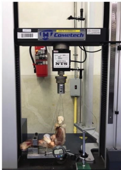
Figure 4 Image of experiment by Pisitwattanaporn et al. [25] where the base of humerus bone was fixed and force was applied
