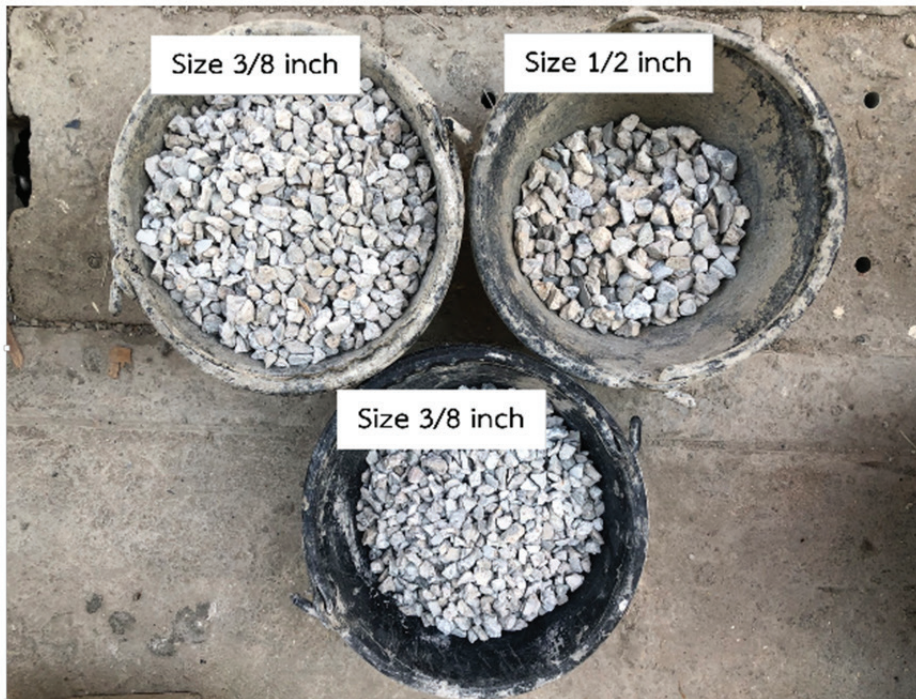
Figure 2 Samples of coarse recycled aggregates used in this work
