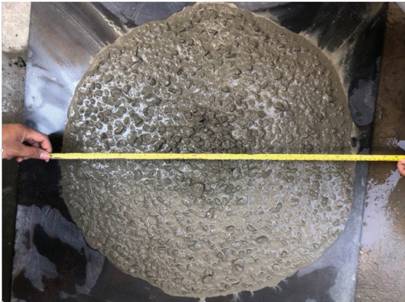
Figure 6 Sample of mixture with slump flow diameter of 75 cm
