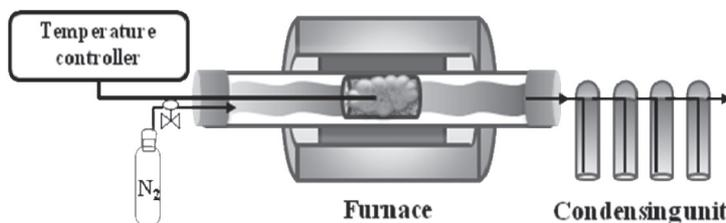
**Fig. 2** Schematic diagram of experimental set-up of pyrolysis experiment
