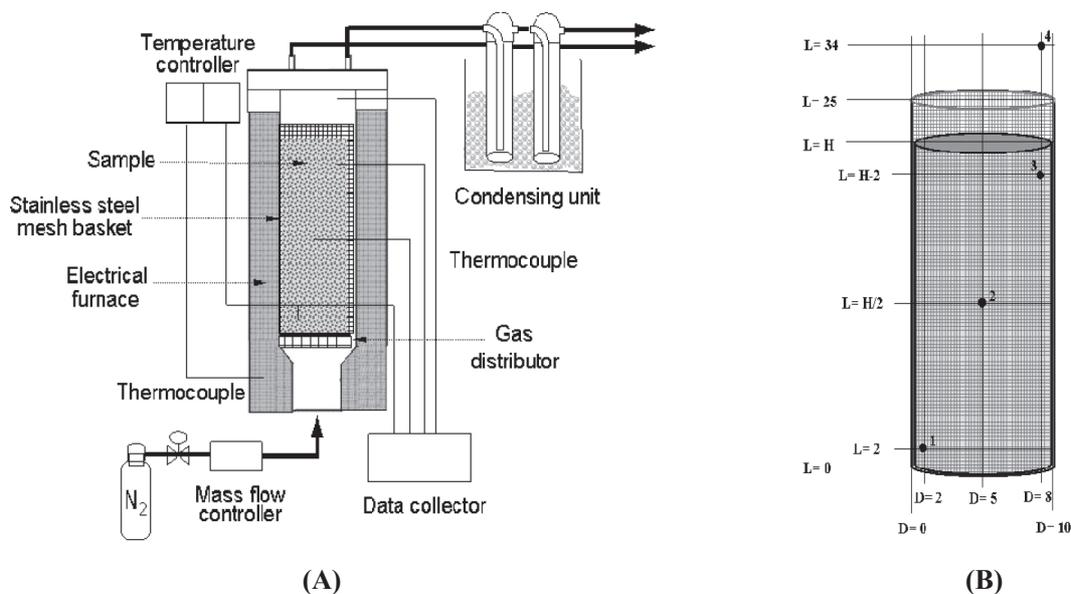
**Fig. 1** (A) Experimental system for torrefaction experiments,
