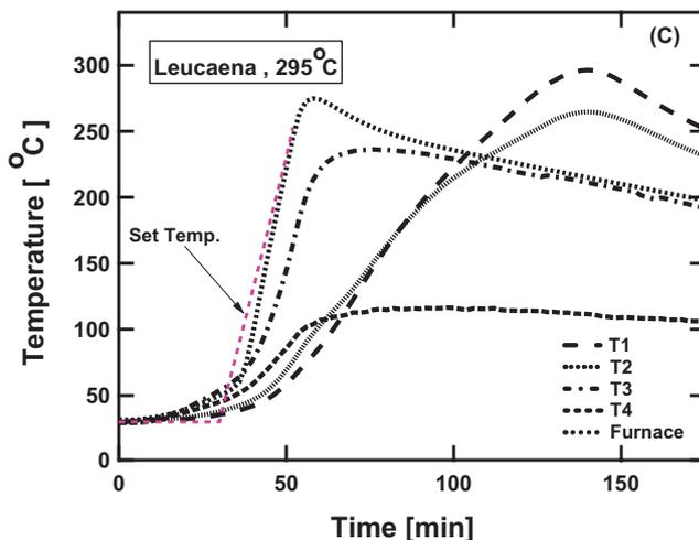
Fig. 3 Temperature profiles during the torrefaction of leucaena at 230°C (A), 260°C (B), and 295°C (C)
