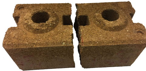
c. Typical failure of brick in splitting tensile test
