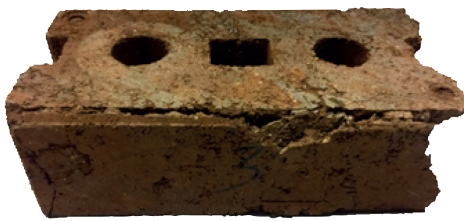
a. Typical failure of brick in compression
