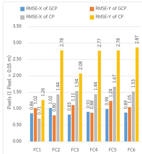
**Figure 4**  $\text{RMSE}_x$  and  $\text{RMSE}_y$  of GCPs and CPs for each flight configuration
