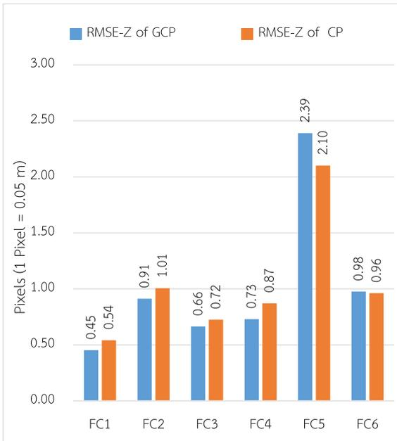
Figure 6 RMSE<sub>Z</sub> of GCPs and CPs for each flight configuration
