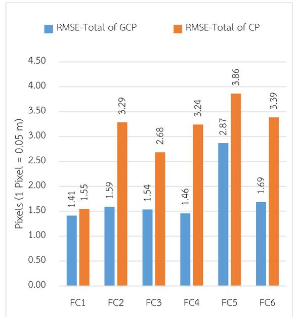
Figure 8 RMSE<sub>T</sub> of GCPs and CPs for each flight configuration
